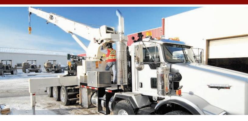
The WHL35TC75 is a natural evolution of our popular 30-ton cranes. Higher lifting capacity and longer reach are obvious benefits of this design. The versatility of integrated out and down outriggers allows for crane set-up in space restricted areas. These cranes have a wider total spread than other outrigger styles and a dual control station design means the crane can be operated from either side.
