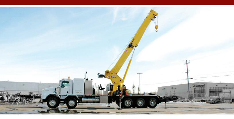
The WHL35TC97 is a natural evolution of our popular 30-ton cranes. Higher lifting capacity and longer reach are obvious benefits of this new design. The versatility of integrated out and down outriggers allows for crane set-up in space restricted areas. These cranes have a wider total spread than other outrigger styles, and a dual control station design means the crane can be operated from either side.
