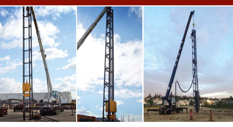
The WHL Pile Driver allows quick and easy conversion your Weldco Hydra-Lift crane application into a pile driver application and vice versa, onsite. The addition of a pile driving hydraulic circuit with heavy duty quick couplers for pressure, return, and case drain, facilitates this quick field conversion of the crane. 55.5 ft leads easily accept 40 ft lengths of standard piling material.
