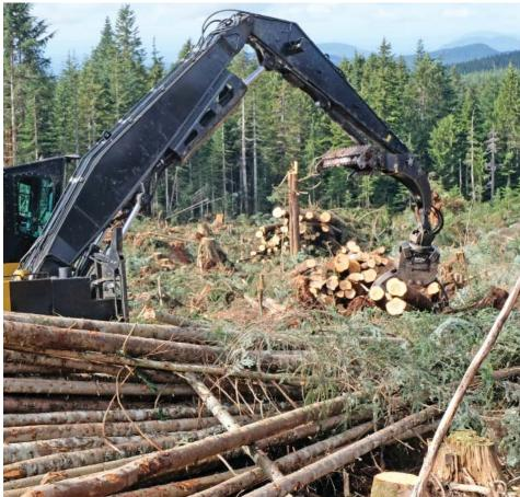
WBM's Heel Grapple is specifically designed for loading, sorting, decking, and hoe-chucking (shovel logging/ forwarding) tree length wood.
