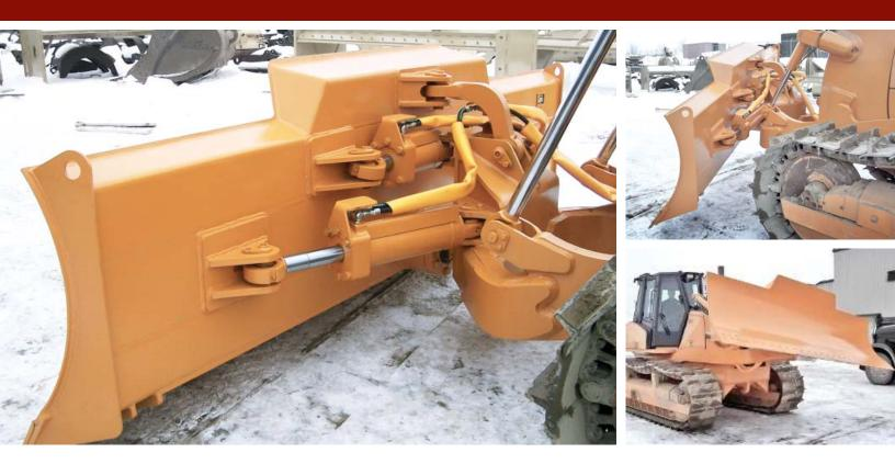
The 6 Way Power Angle/Tilt Blade adds versatility to your Crawler Dozer. Set your blade for grading, trimming, sloping, ditching, or a variety of other tasks without leaving your cab. Designed and built to last with years of proven service in the field, a WBM 6 Way Blade is a powerful attachment for your Crawler Dozer.
