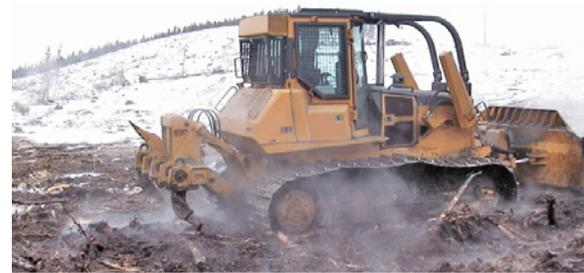
WBM Rippers are used to 'rip' or break up compacted or frozen ground conditions to enable easier grading, dozing or stockpiling operations to take place.
