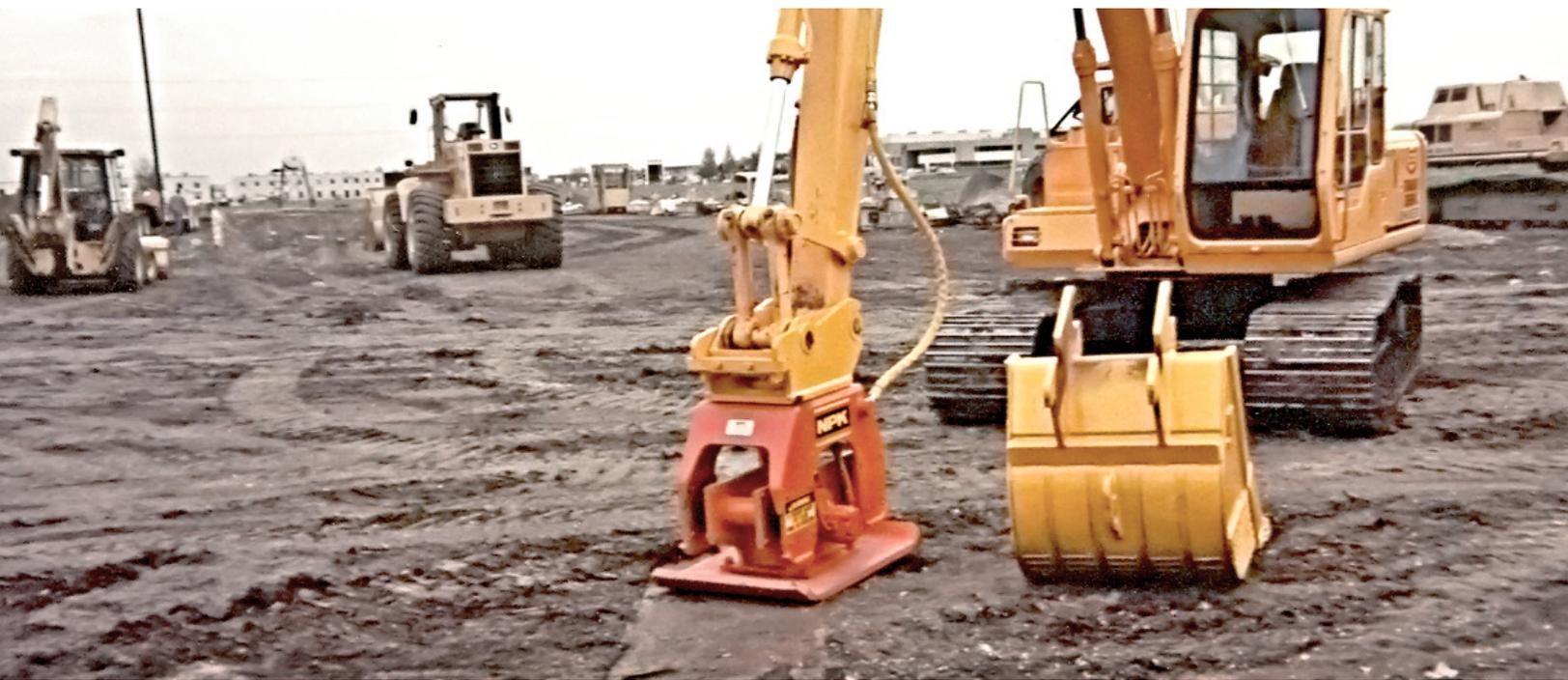
WBM's Compactor/Hammer Adapter enables users to easily change a variety of hammers, compactors, augers and other tools to the Coupler System.
