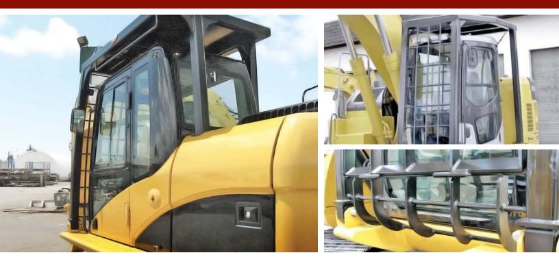
WBM's FOPS (Falling Object Protection Systems) are designed to protect the excavator cab and operator from falling objects in dangerous environments. FOPS are used primarily in the demolition, forestry and construction industries.
