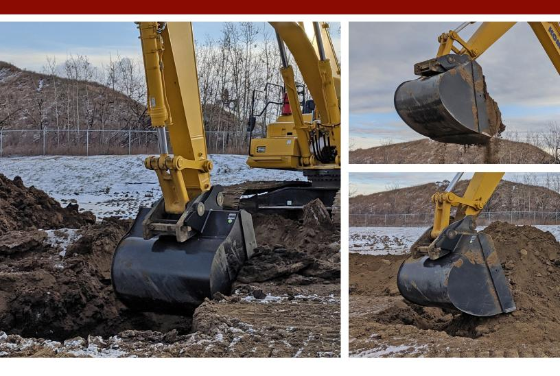
WBM's Manual Wedge Coupler enables quick changes between attachments that are WBM quick coupler lugged on machine models within the same weight class.
