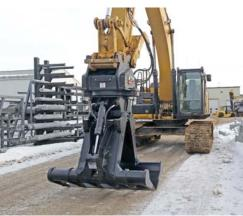
The WBM Mat Grapple is designed to play the critical role of removing and placing rig mats, used to extend the drilling season and to protect the environment.
