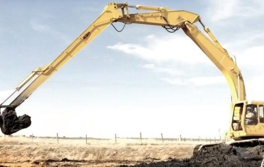
A Quick Extension Stick is an excellent addition to an excavator that provides users with extended reach on their existing boom and stick. It enables users to utilize their conventional excavator as a long front excavator and then easily change back to a conventional front.
