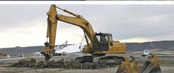
The WBM Stick Mounted Ripper is ideal for digging into frost, rocky soil or shale to enable easier excavation of material.
