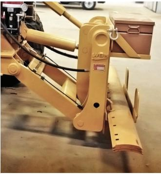
WBM Cutting Edge Rack with Toolbox provides safe and easy storage of replacement grader moldboard bolt on edges, tools, and spare parts.
