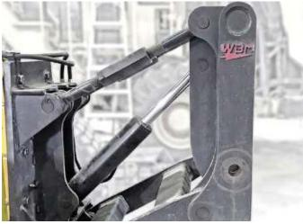
The WBM Motor Grader KAT (Kwik-a-Tach) Master Hitch Lift Group is a quick and convenient way of switching attachments on a Motor Grader. Attachments that are lugged with WBM quick coupler lugging can be either hydraulically or manually attached within minutes.
