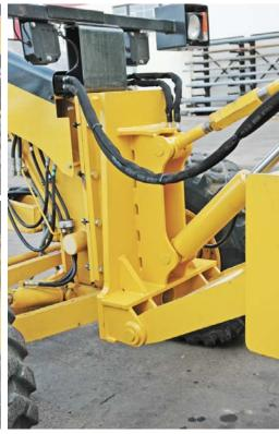
The WBM Integral Lift Group utilizes a direct pin-on connection between the attachment and lift group linkage. This lift group is an economical alternative to the KAT Master Hitch lift group system.
