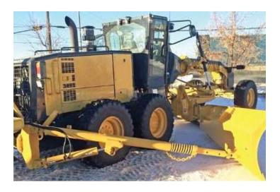
A Standard Wing requires two sets of proportionally actuated machine auxiliary hydraulics (2750-2500 psi @ 10-30 gpm).
