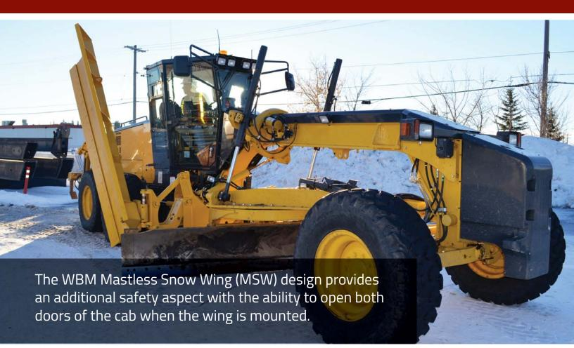
Mechanical and Hydraulic float at the discharge (toe) and mechanical float at the intake (heel) of the moldboard give an increased life cycle and easier operator usage when experiencing uneven or rough terrain. The MSW's compact design significantly improves the grader's blade angle during operation, allowing for full machine articulation.
