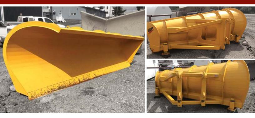
WBM Motor Grader One Way Plows are used exclusively for clearing snow. The funnel-shaped, radial moldboard profile easily and effectively clears and casts snow. Operating the grader at moderate to high speed forces the snow into the tight curvature of the moldboard, which funnels it up and out of the large radius open end.
