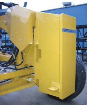
WBM Motor Grader Push Block/Counter Weights have a dual purpose on Motor Graders. As a push block, the attachment acts to protect the front of the grader when pushing other machines. This attachment will also increase traction of the front wheels, if the grader is equipped with front wheel drive, and increase steering capability when grading.
