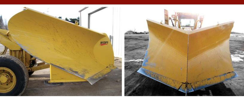
WBM V-Plows are designed for initial path clearing on snow-drifted roads. The unique 'V' shape provides a wedge action to breakup hard-packed snow and cast it to the sides of the grader. The aggressive curvature allows snow to be rolled and discharged quicker and further, while forcing the blade to carry less snow during operation.
