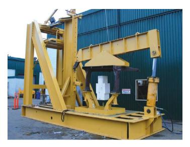
Our Structural Performance Test Stand is used to prove design and engineering necessary to meet rigid industry standards. Protective structures can be tested to ISO, SAE, OSHA, CSA, ANSI, WCB, BSI, CEN, and various other specific standards.
