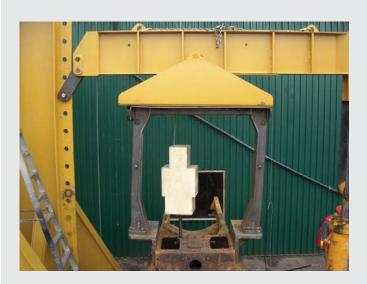
To maintain compliance with rigid standards, our computer analysis determines the stress level of each section of the roll-over protective structure. Prior to release for manufacture, all ROPS prototypes are tested to failure on our Structural Performance Test Stand. Protective structures can be tested to ISO, SAE, OSHA, CSA, ANSI, WCB, BSI, CEN, and various other specific standards.
