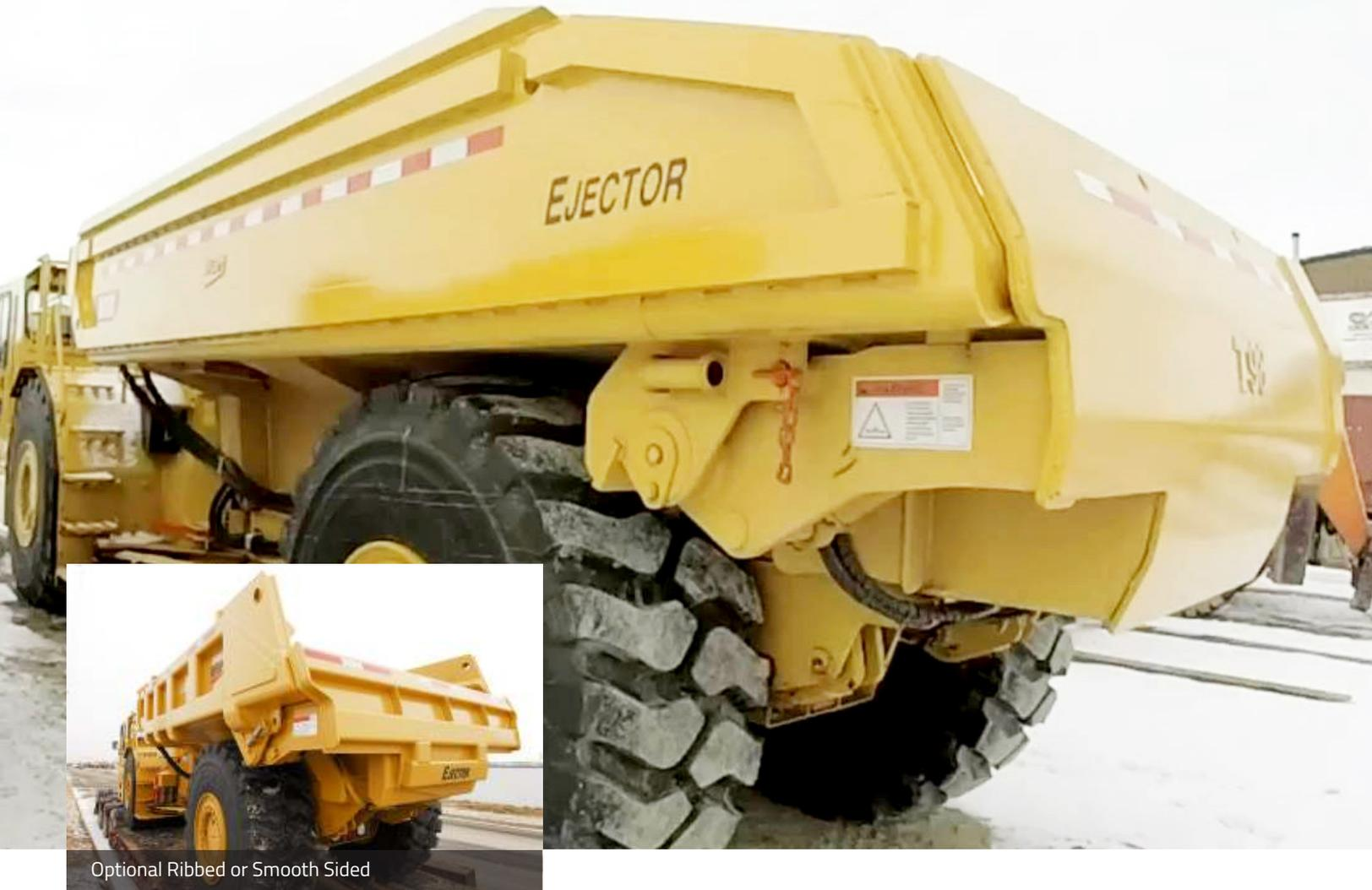
WBM's Underground Ejector Bodies make articulated trucks ideally suited for operations in areas with limited overhead clearance. Being able to discharge the full load without having to raise the body, Ejector Bodies offer greater stability particularly on soft surfaces.
