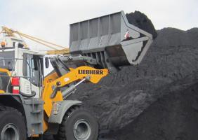
WBM Coal Buckets are used to load hoppers, conveyors, trucks or train cars from mined or loose coal stockpiles. Due to increased payload expectancy, WBM Coal Stockpiling buckets are typically 15-20% larger in capacity then Coal Seam buckets.
