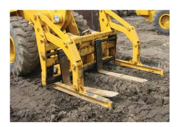
Pipe and Pole Fork Racks with Dual Top Clamps provide all of the same features as a standard Pipe and Pole Fork Rack with the added feature of dual over arms that clamp and stabilize the load in position. This type of Fork Rack is used extensively in pipe yards for carrying and loading pipe of various lengths and diameters.
