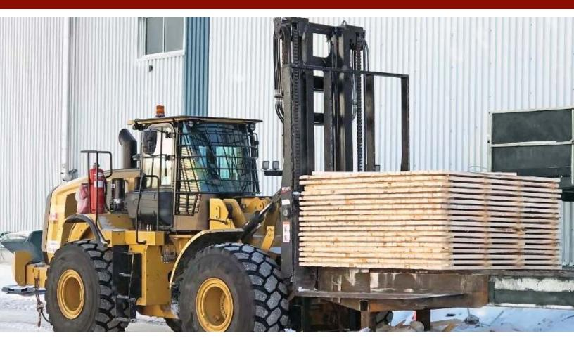
WBM's Heavy Duty Forklift Masts are designed for conversion of wheel loaders for rough terrain forklift applications.
