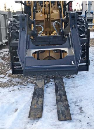
The improved "Max-View" WBM Mat Grapple for wheel loaders is used to remove and place mats, which protect the environment and extend the construction season. This enables safe access for crews and heavy equipment.
