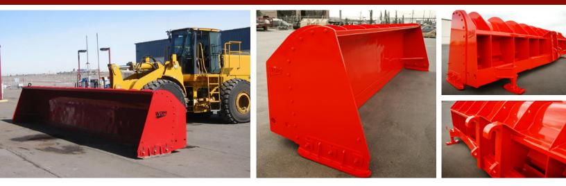
WBM Runway Plows are used for clearing snow from airport runways and parking lots. They are available in a "straight blade" design, manufactured in 5' increments starting at 15' up to 30'. Ramp Hogs utilize bolt-on wings on each end of the blade to eliminate windrows and an optional rubber flap bolted to the top of the blade to decrease 'blow-over' of snow that affects operator visibility during high speed clearing.
