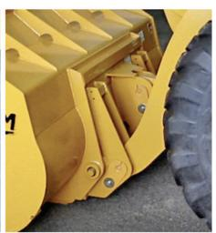
WBM WLKAT (Wheel Loader Kwik-a-Tach) Series Master Hitch is an innovation design that increases the versatility of the Wheel Loader.
