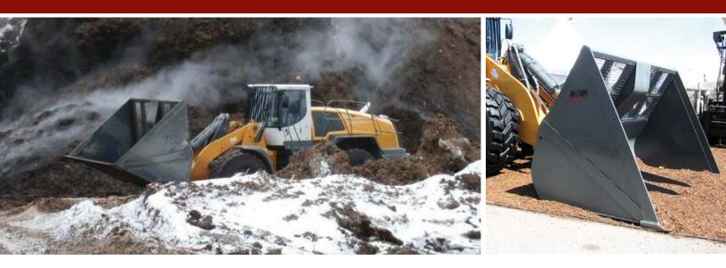
WBM Woodchip Buckets are the largest of the Light Material Buckets. Due to the lightweight nature of woodchips, this style of bucket is designed to handle very large capacities. The WBM design addresses the issues of machine stability, bellcrank interference and operator visibility.
