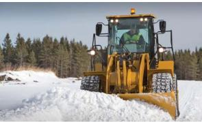
WBM U/V Angling Blade is a versatile blade used in snow removal applications. The moldboard is hydraulically configured to U-Style, V-Style, Straight or Angled blade types.
