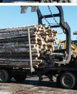
WBM's High Capacity Cut-to-Length Grapples (formerly known as Pelican Grapples) are designed for single pass loading/unloading in barge and mill yard applications.
