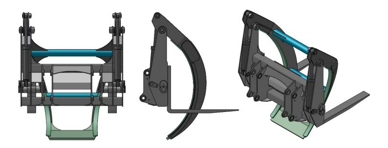
WBM Log and Lumber Forks are designed with both fork and grapple characteristics. With a hook type profile and heavy duty box construction, the overarm provides excellent stability and holding characteristics when handling tree length or short wood. When overarm is opened, the forks enable lifts of lumber to be handled without interference.
