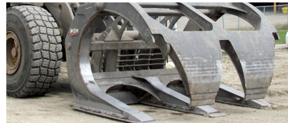
3-tine grapple shown with extra bottom wear plate and split overarm (clamp)
