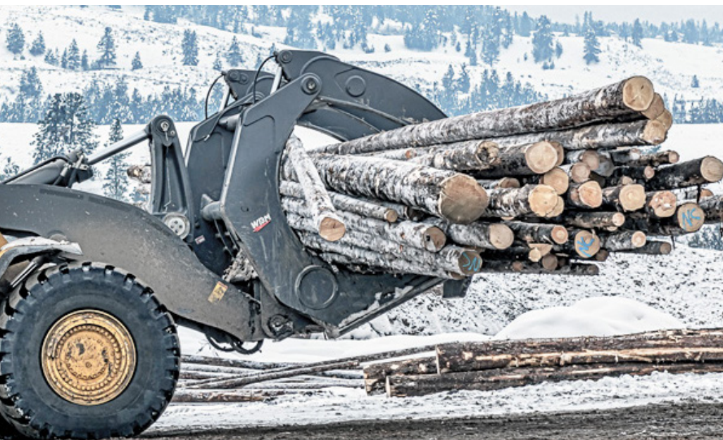
3-tine grapple shown with extra bottom wear plate and split overarm (clamp)
