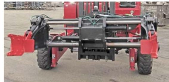
WBM Tire Handlers are designed to safely and efficiently handle OTR tires. The TH3 is a fully integrated, turnkey rough terrain / short wheel base tire handler; ideal for underground mines, construction sites and mobile tire service (12:00R24 – 29.5R29). Based on Sellick STM70 carrier machine.
