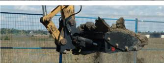
The WBM Chuck Blade is designed to move more material in less time than a conventional bucket. It has a 45° hydraulic tilt and is commonly used for clean-up and sloping, canals, pipeline, pavement stripping, basement work and cement slab preparation.
