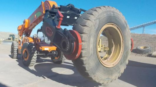
WBM W series Tire Handlers are designed to safely and efficiently handle OTR tires and rim assemblies on large mobile equipment.
