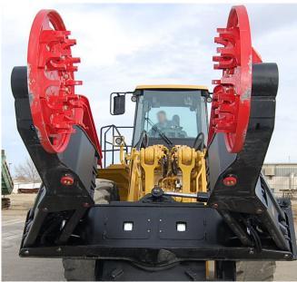
WBM C series Tire Handlers are designed to safely and efficiently handle OTR tires and rim assemblies on small to medium size ADT's, OHT and mobile equipment.
