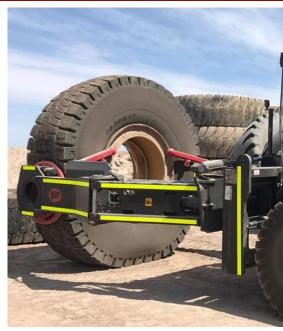
WBM W series Tire Handlers are designed to safely and efficiently handle OTR tires and rim assemblies on large mobile equipment.
