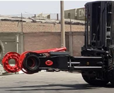
WBM - W series Tire Handlers are designed to safely and efficiently handle OTR tires and rim assemblies on large mobile equipment.
