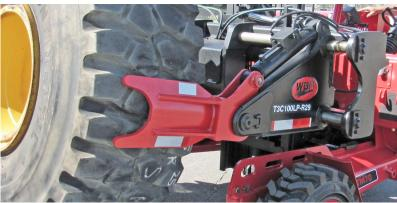
WBM C series Tire Handlers are designed to safely and efficiently handle OTR tires and wheel assemblies on underground and small surface mobile equipment.
