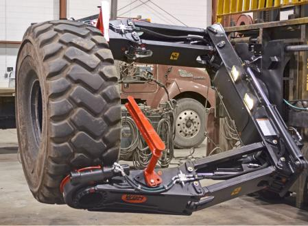
WBM W Series Tire Handlers are designed to safely and efficiently handle OTR tires and rim assemblies on large mobile equipment.
