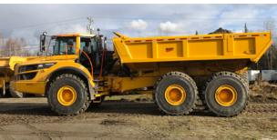
WBM's Ejector Bodies utilize dual cylinders, which push the material out without raising the body. This articulated truck modification is an effective replacement for traditional dump style bodies in situations where overhead clearance is restricted and/or the ground is uneven.
