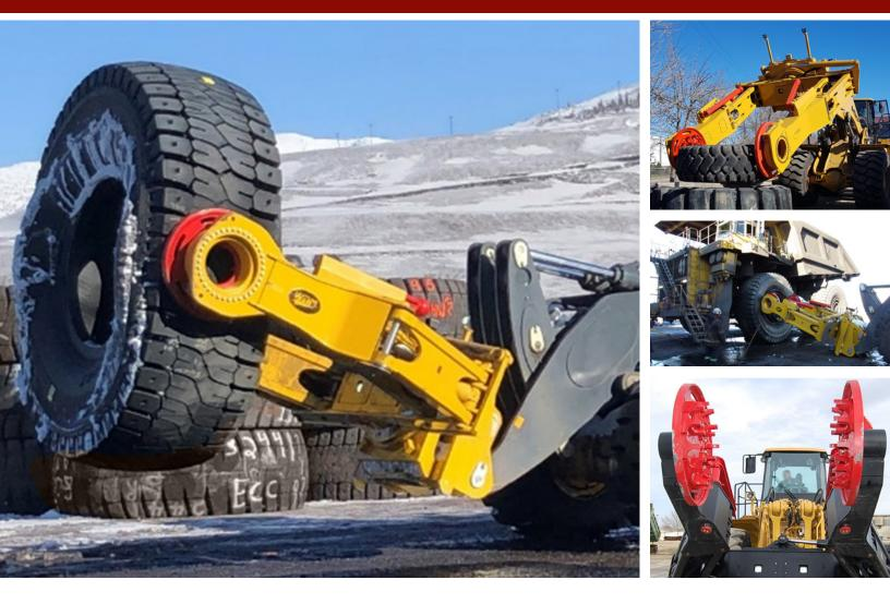
WBM Tire Handlers are designed to safely and efficiently handle OTR tires and rim assemblies on large mobile equipment.
