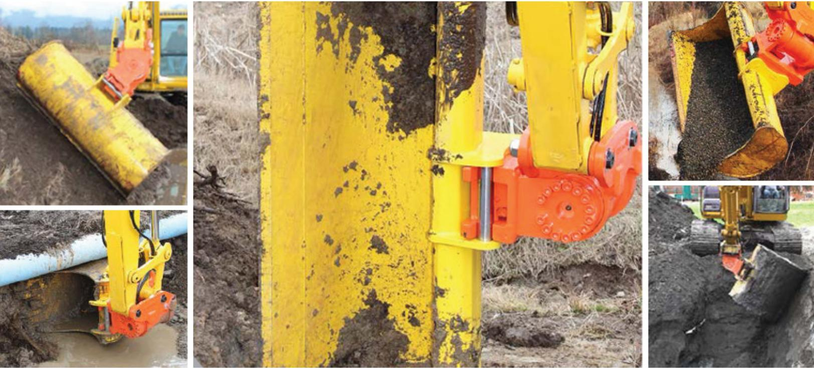
The Weldco-Beales Manufacturing Powertilt Coupler increases the capabilities of any quick coupled attachment. Working as a tilting coupler, the Powertilt Coupler can rotate attachments up to 180°, making it ideal for sloped trenching, excavating around foundations and sidewalks, and ditch cleaning.
