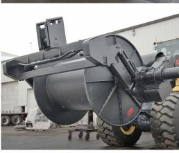
The WBM (High Capacity) Cable Reeler CR600/1000 Series are designed to safely and efficiently handle the distribution and trailing cables for electric powered equipment in underground or open pit mines.
