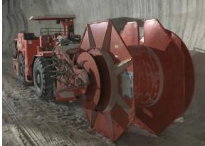
WBM Cable Reeler's are designed to handle electric distribution and tailing cable used in open pit and underground mines around the globe.
