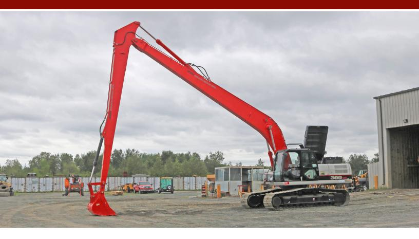
WBM Long Reach Fronts are designed and manufactured to support deep and long-distance digging applications, such as: dredging, canal cleaning, lagoon cleaning, material handling, river and canal pipeline crossings. WBM Long reach Fronts are available in either a Dredging configuration (Super Long Reach), or an Excavating configuration (Long Reach).
