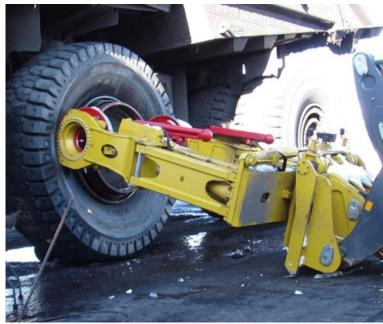
WBM W series Tire Handlers are designed to safely and efficiently handle OTR tires and rim assemblies on large mobile equipment.
